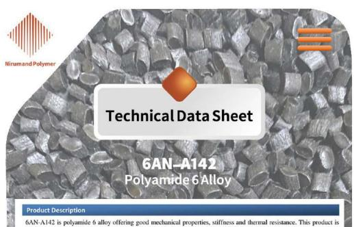
6AN-A142 is polyamide 6 alloy offering good mechanical properties, stiffness and thermal resistance. This product is used in automotive applications and other utility products. This grade is designed to be processed in conventional injection molding process.
